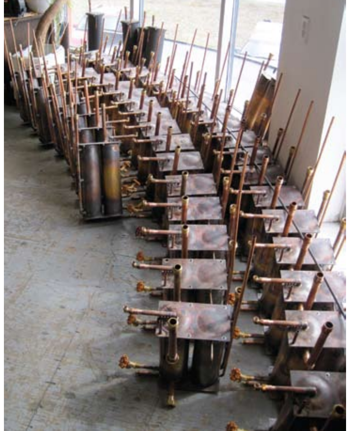
Copper heat exchanger units with connections installed await final assembly into their protective orange enclosures.
