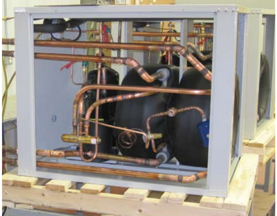
An interior of a module showing the range of copper tube sizes used.
