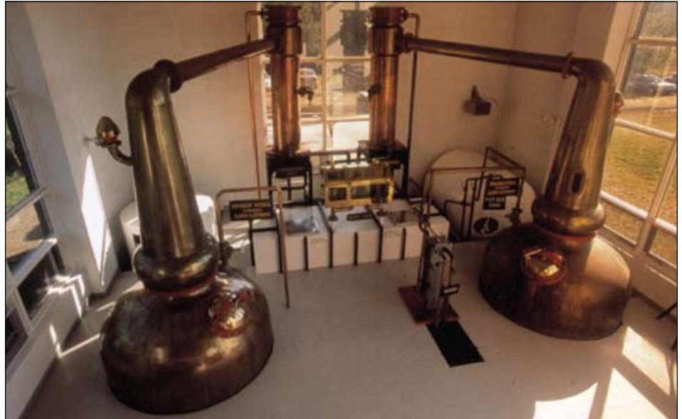
Copper spirit and wash stills, originally made by Forsyths Coppersmiths.
