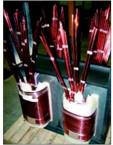
Copper magnet wire is used for the windings of transformers.
