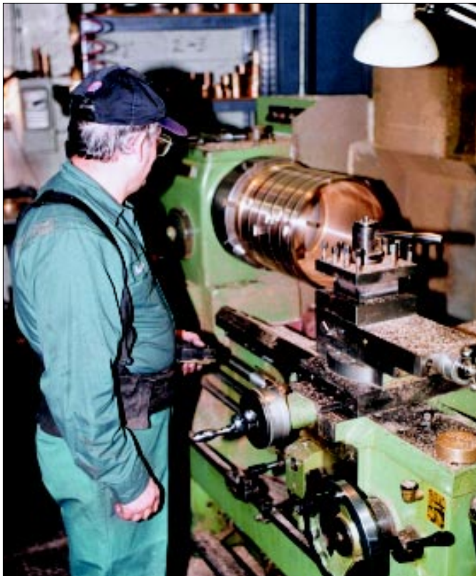
Machining a large bearing at K.P. Bronze.
