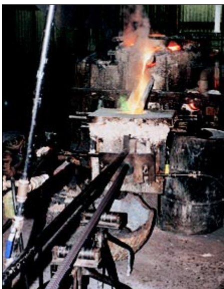
Continuous casting of hexagonal bronze bar.
