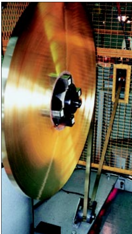
C26000 brass strip in coil form is fed from the feed spool into the roll forming portion of the production line.
