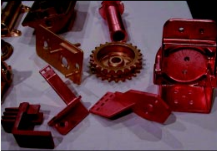
A selection of copper based parts made by the permanent mold process.
