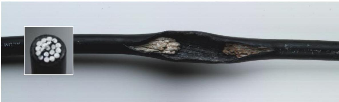
*Failed aluminum cable from water corrosion*
